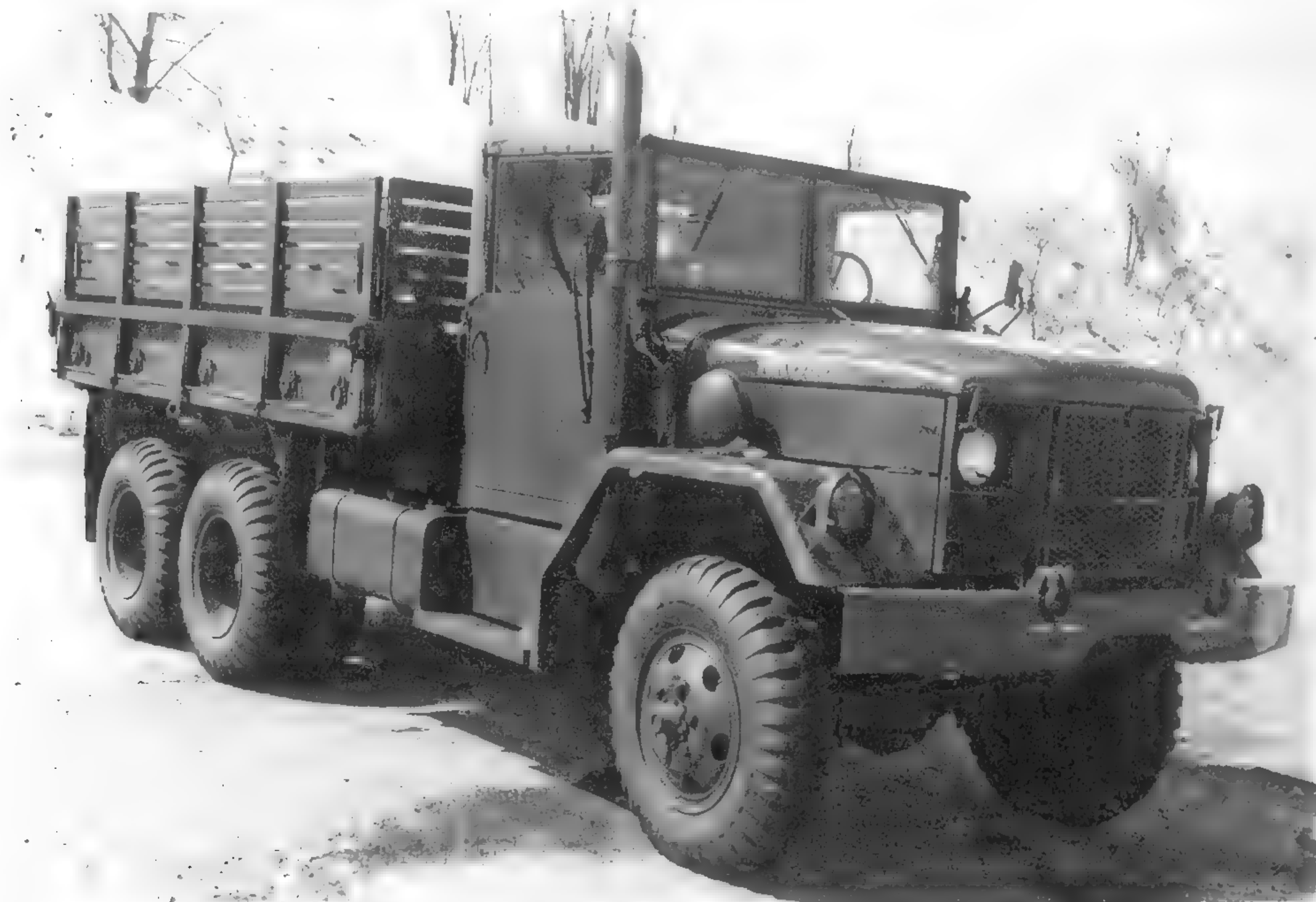
A Multifuel engine also powered the M35A2 and M35A2C (drop side, shown here), this time an LDT-465 version. Various exhaust systems were used horizontal muffled, vertical muffled, and vertical non-muffled. The non-muffled exhaust was used with the turbosupercharged engine. (U.S. Army photo)
